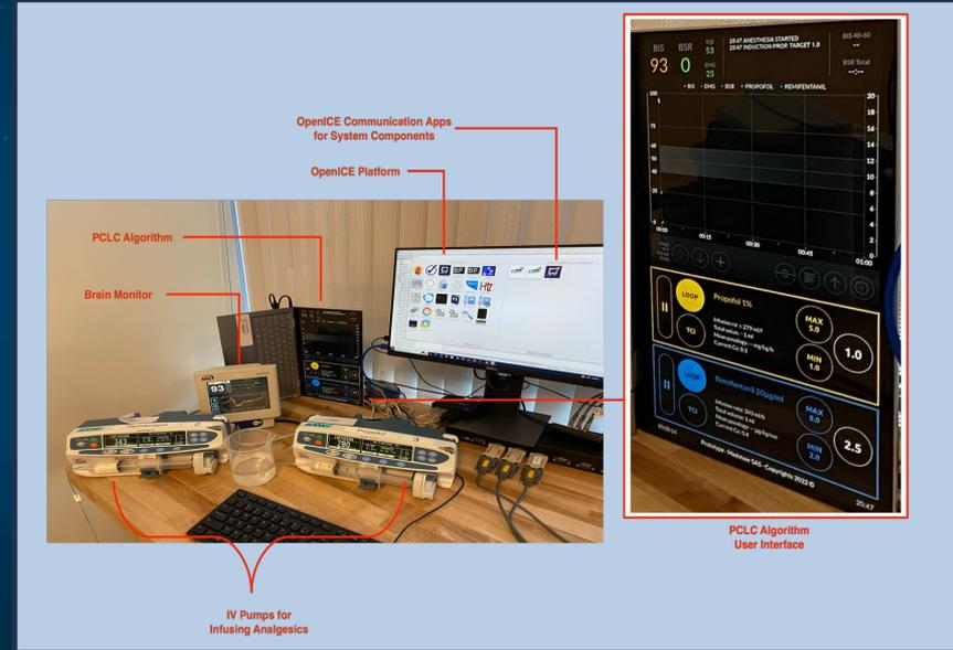
OpenICE-based hardware-in-the-loop testbed for a PCLC anesthesia system
