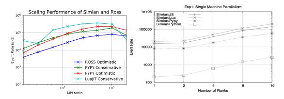
Figure 2: Performance of Simian platform against Ross from 4 to 2048 cores. Lua has the best performance from 16 to 1024 cores. Lua also outperforms JavaScript and Python.
