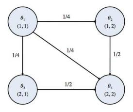
**Fig. 3.** Rate matrix  $A: \theta_1$  is the normal operating state. The entire system can fail and transition to another mode at equal rates to  $\theta_1, \theta_2, \theta_3$ . The intermediate failure modes  $\theta_2, \theta_3$  switch to  $\theta_4$  when cyber attack occurs.  $\theta_4$  is the absorbing state. The system can not recover immediately once damaged.
