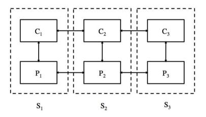
**Fig. 1.** Three interconnected CPSs: Each system  $S_j$ , j = 1, 2, 3, is composed of its cyber system  $C_j$  and physical system  $P_j$ . Three CPSs have interactions at both the physical layer and the cyber layer.
