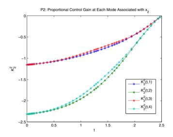
Fig. 5. Individual feedback control term of  $P_2$  with respect to state  $x_2$
